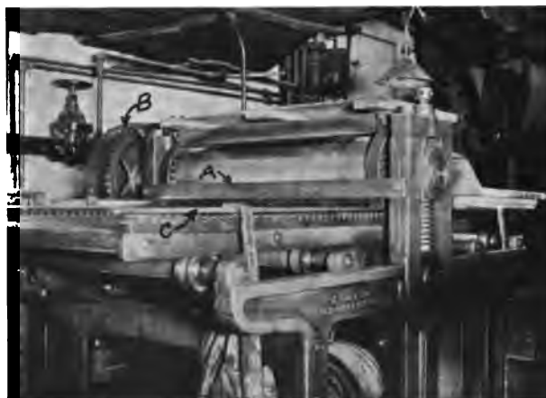
Fig. 5. Guards for Matrix Roll (A), Gear (B) and Rack (C) of Press.†
